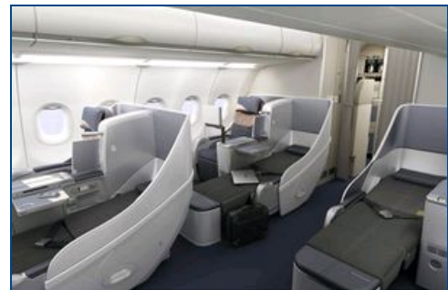
Shown above is the 2x2 arrangement of the lie-flat beds in a specially configured Airbus A318.
